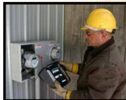
Meter testing is being done on this dual fuel meter after the implementation of the automated meter reading system.
