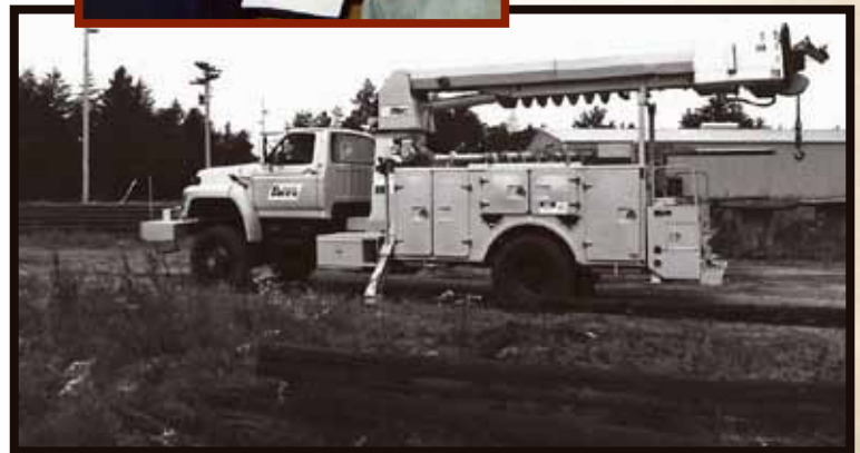
This digger-derrick truck is used in boring holes and setting new poles. It is also used as a crane for heavy lifting. The cab and chassis is a 1988 Ford F800D with a 7.8 liter diesel engine.
