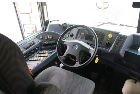
The driver's seat and bus interior. At right is the charging display, which shows the battery percentage and energy usage.
